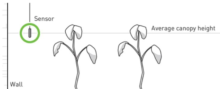
If you are using another climate control system, hang it close to the sensor of that system. If necessary, the sensor cable may be lengthened an extra 5 meter with a standard 3.5 mm jack extension cable. A sensor with a cable length of 30 meter is also available.
